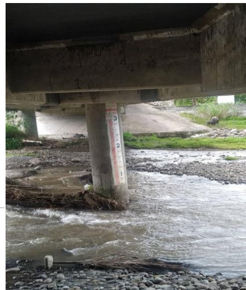
Conventional Stage gauge water level Monitoring ( OLD SYSTEM )
